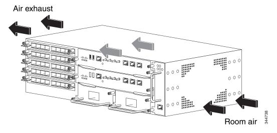
The fan trays maintain acceptable operating temperatures for the internal components by drawing in cool air through the vents, and circulating the air through the chassis.
